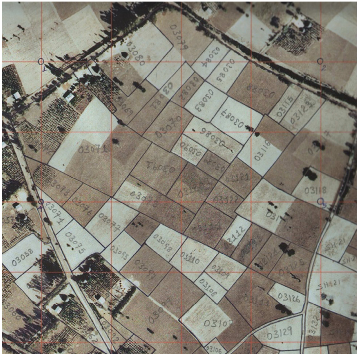
Figure 2. Orthophoto used as a field work map sheet with a georeferenced grid. The map shows the delineated parcel boundaries and parcel identification numbers (Ethiopia).
